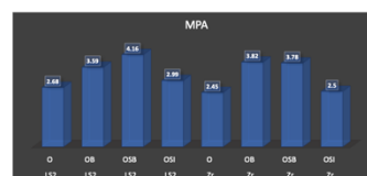
Figure 7. Maximum shear stress of cement
