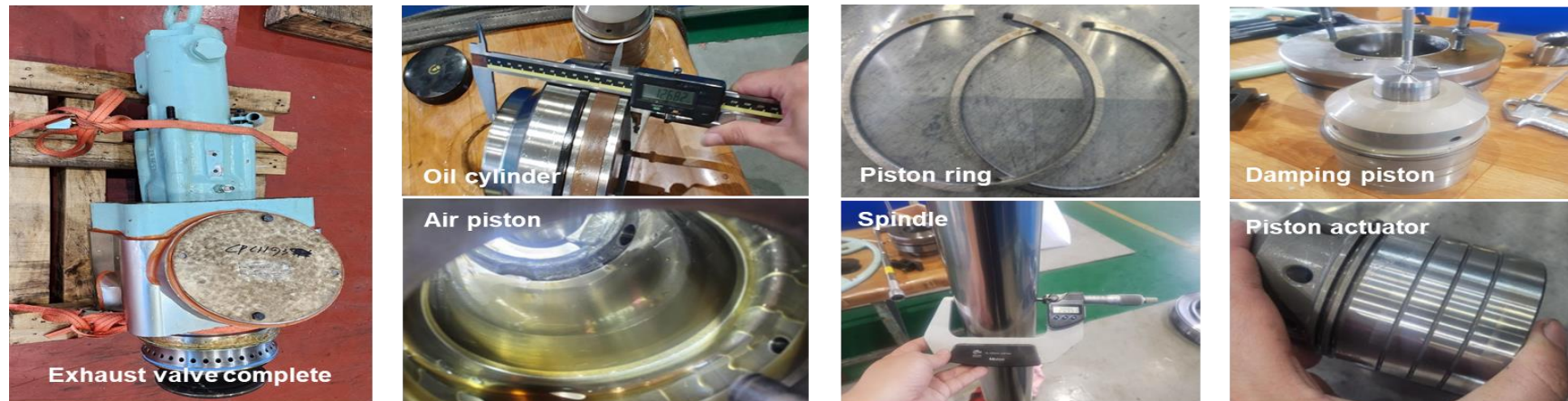
[ Inspection of exhaust valve components ]
