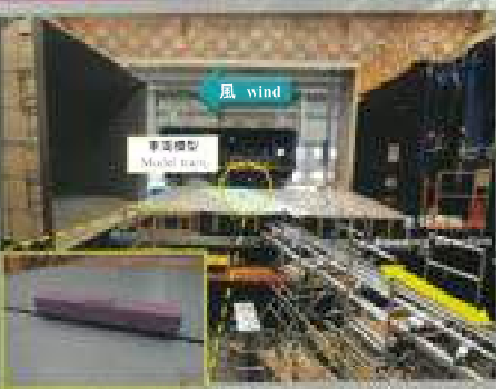
横風を受ける車両の風洞試験 Cross wind test in the wind tunnel using a running model train
