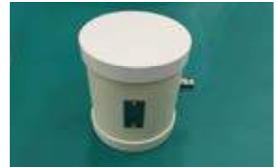
Horn Antenna (used for VRS antenna)
