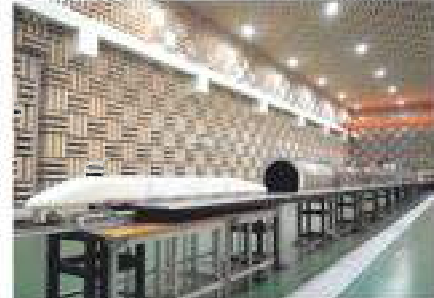
低騒音列車模型走行試験装置 Low-noise moving model test facility
