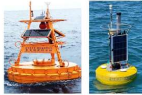
Real-time, long-term ocean & atmosphere monitoring in open ocean by moorings
