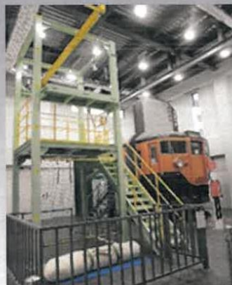
Experiencing an accidental fall (sandbag drop and try out of safety belt)
