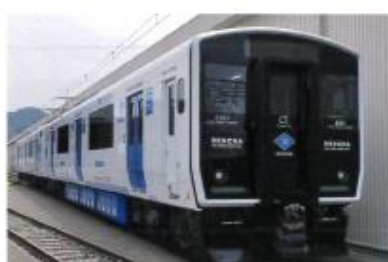
九州旅客鉄道 株式会社股納 BEC819系交流架線式蓄電池電車 Series BEC819 AC-electrified dual energy charge train for Kyushu Railway Company.
