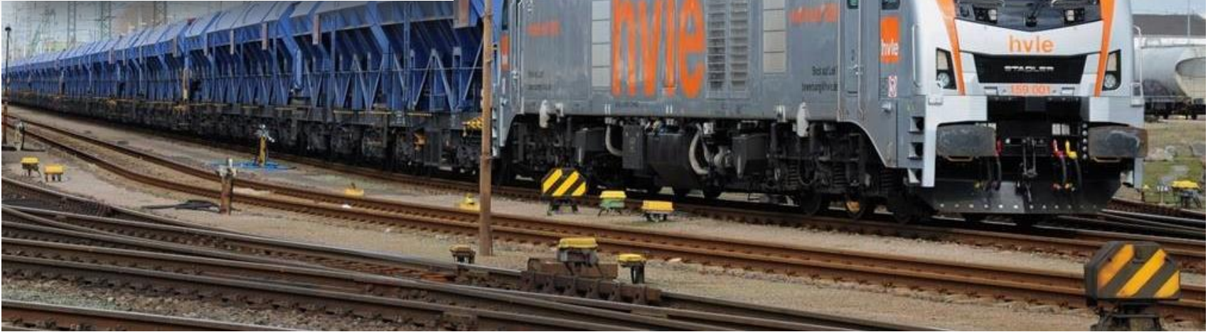
1. HVLE (Germany) Locomotive in the Rübelandbahn(德國)Rübelandbahn的HVLE機車 Operations on up to 64‰ ramps於高達 64‰ 的坡道上行駛
