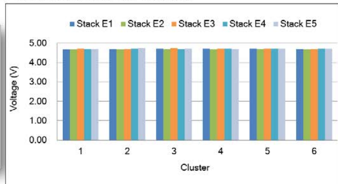
Voltage distributions of power output at 1.2 kW for stack E1~E5 at 700 °C
