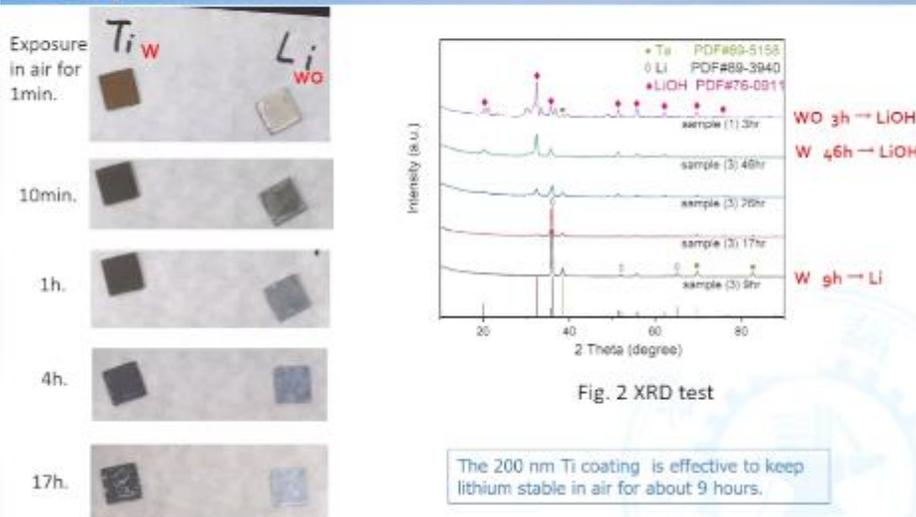
Fig. 1 Exposure and scratch test
