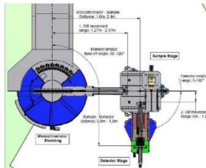
Proposed design of neutron powder diffraction instrument
