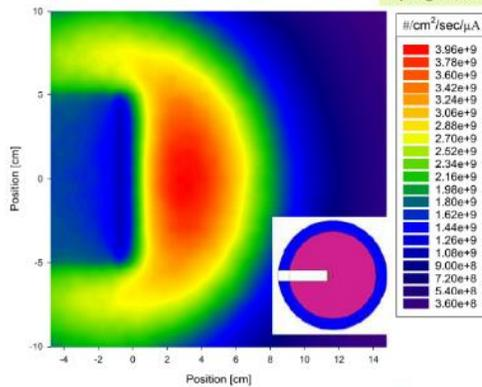
Thermal neutron flux distribution for 70 MeV/1mA proton beam.
