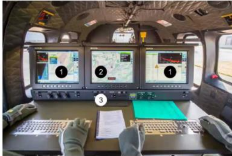
Figure 2: Operator console of the RLL system. 1. Displays of the client computers. 2. Common display (mirrored in the cockpit). 3. Control panel with switches for power, lighting and communication and USB ports for file exchange.
