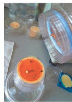
After density separation in a funnel, samples are transferred to polycarbonate filters.
