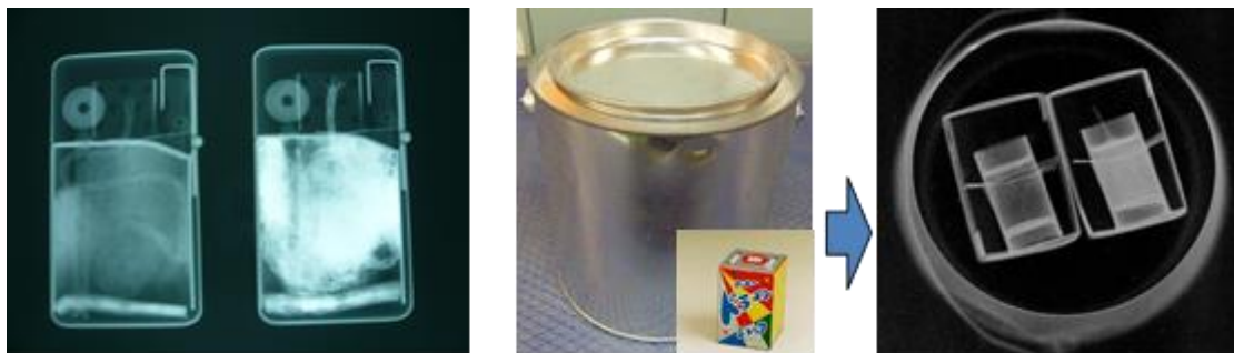
Observation of oil in oil lighter (Left : none Right : Remanent)
