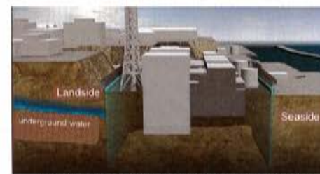
Image showing how to block the inflow of underground water into Units 1-4
