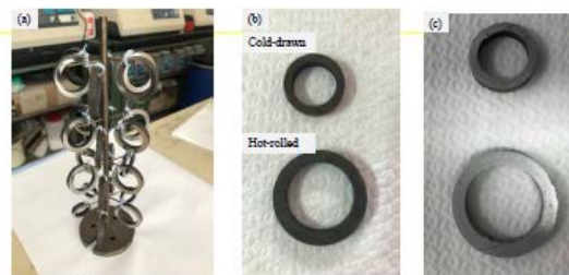
Figure 2 (a) Before corrosion test specimens and after corrosion specimen (b) before cleaning (c) after cleaning
