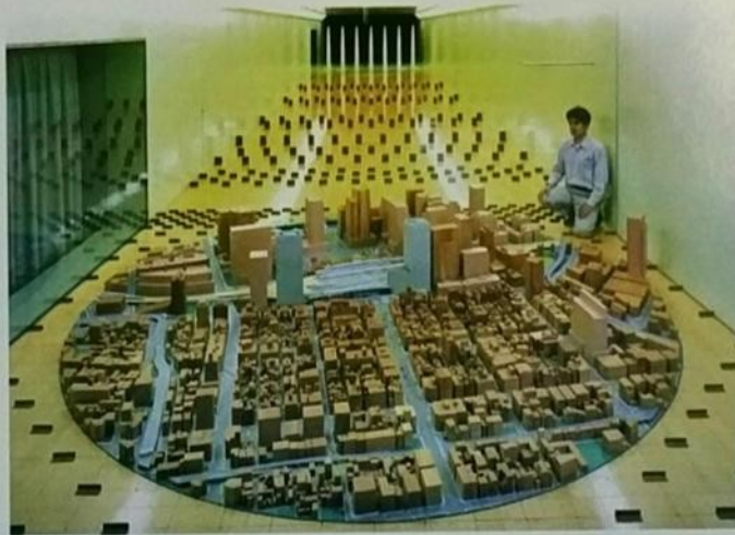
市街地模型を用いた超高層建築物の風圧測定 Wind Pressure Measurement of a High-rise Building with an Urban Model
