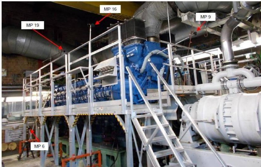
Installation of the 20V 8000 M71L in test cell 130 with indication of microphone positions
