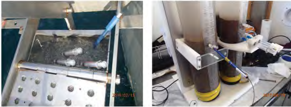
Fig. 1. Extraction of pore-water from grab and core samples using RhizoCera/syringe samplers. Dissolved oxygen (right) and redox (left) probes are also shown.
