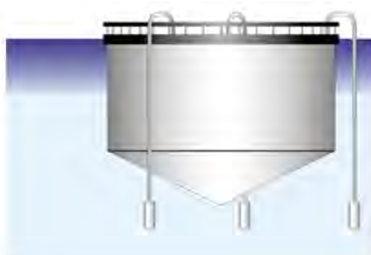
Fig 1. Sketch describing the principle of semi-closed containment with water inlet deeper than the lice belt (purple) (Illustration: Oddvar Dahl)
