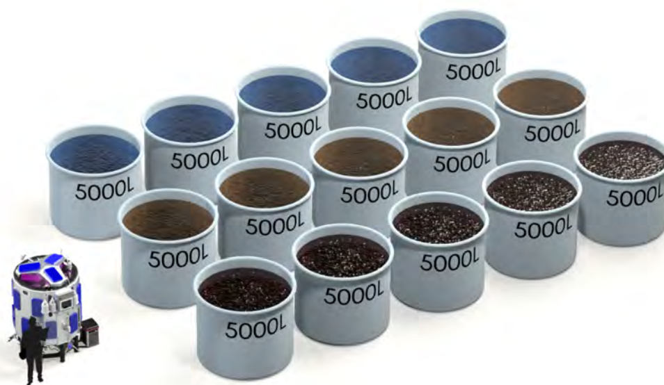
Fig. 1. Equivalent Algal production from PBR 1250L and 75,000L of traditional fiberglass batch tanks growing Thalassiosira pseudonana
