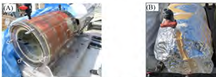
Fig. 1. Photographs of the dynamic aging apparatus. (A): the cylinder with test plates fixed on it, and (B): the cylinder with a light shielding sheet while aging.
