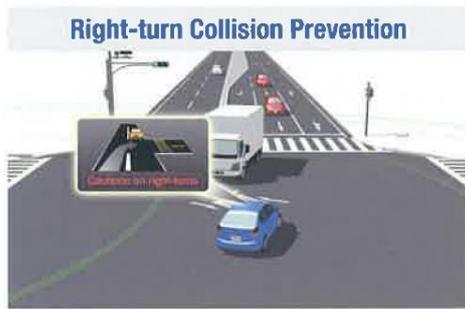
Providing voice messages or images to warn the driver based on oncoming vehicles information supports avoidance of collision when turning right at intersections
