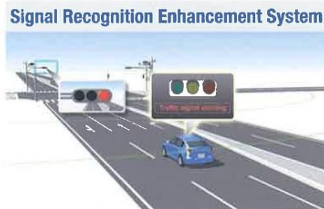
Providing voice messages or images to warn the driver based on signal information supports avoidance of missing red light signal
