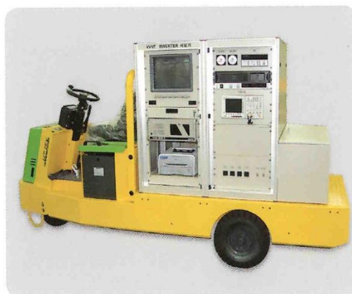
牵引逆变器测试设备 Test Equipment for VVVF Inverter
