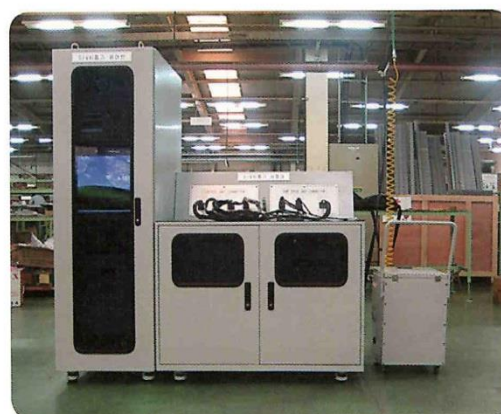
SIV试验机 Test Equipment for SIV
