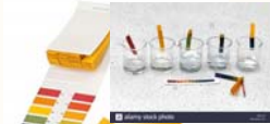
pH paper Dip pH paper into the sample than match the color of you pH paper with the chart
