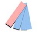
litmus paper if the color of paper changed from blue to red ->acid from red to blue ->base no change -> neutral
