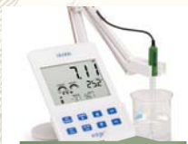
pH meter pH meter would give you a number of 0-14
