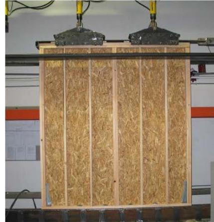
Combined Shear and Wind Uplift Test
