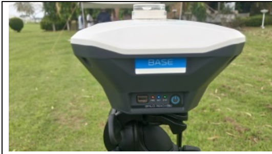
圖7、衛星地位系統Ground control Point (GCP) 搭配之Base
