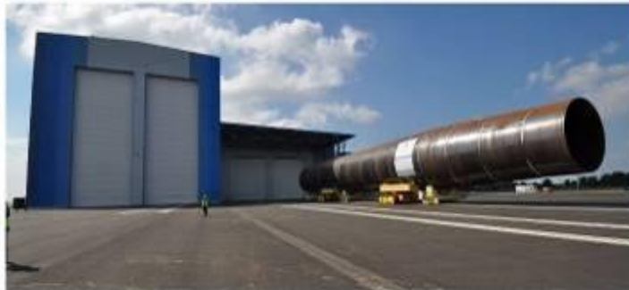
Mega-MonoPile: Diameter 7.8m, Length 63 m, Weight 891 t
