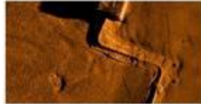
Cable exposures and freespans
