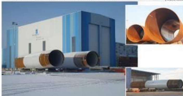
91 MPs: Diameter 5.8m-7.0m, Length 40m - 59m, Weight 435t-650t
