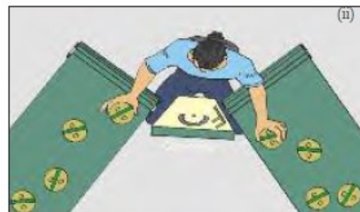
Figure 5c. (i) and (ii) Provide a layout that allows the worker to move objects from one conveyor to the next while keeping a natural posture. Using a transfer plate and rollers makes it easier to move objects.
