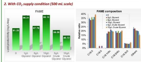
Figure 3. The lipid production of *C. orbicularis* CPC1215 under different concentrations of pure glycerol or crude glycerol in 500 mL PBR with CO<sub>2</sub> supply (5% CO<sub>2</sub>, 0.2 vvm).
