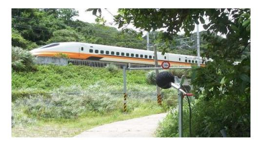
The monitoring of noise from of a passing Taiwan High Speed train
