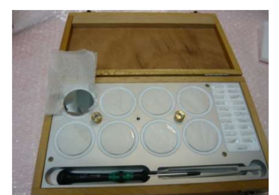
1 kg stack of 8 Pt-Ir disks fabricated at the BIPM
