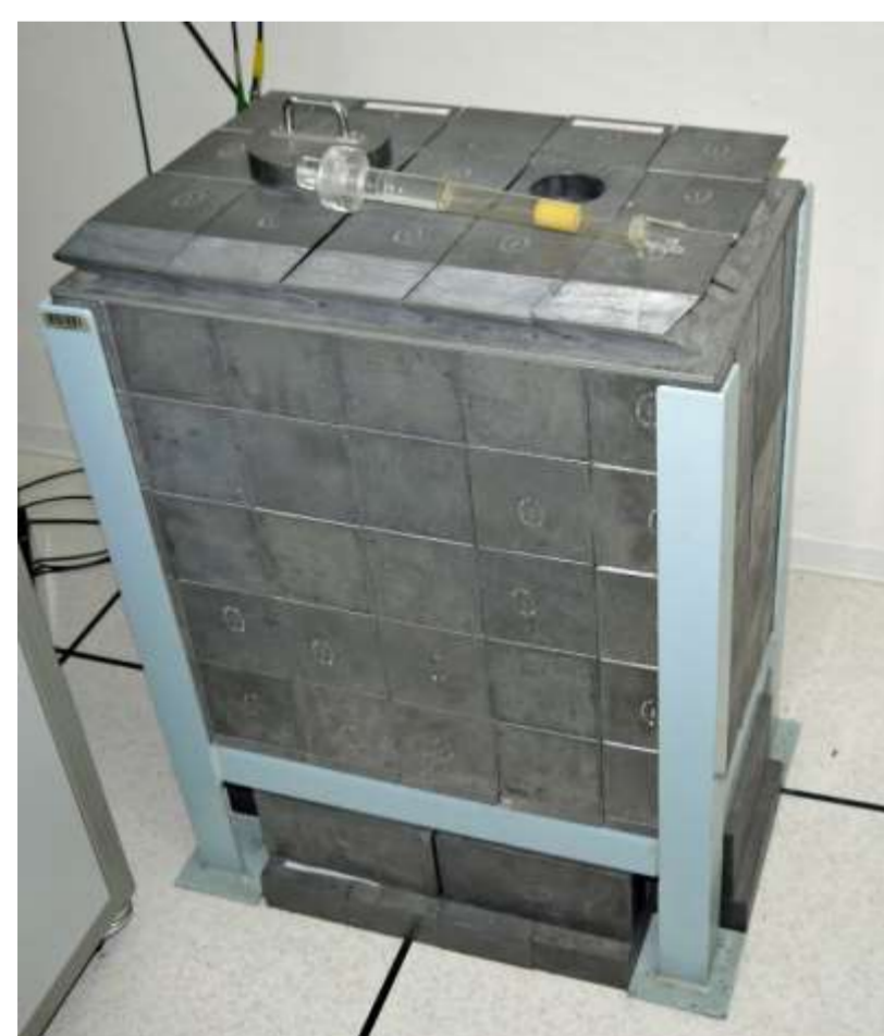
The SIR international reference system enables NMIs to compare standards of gamma-emitting radionuclides, including a comparison of ^{241}\text{Am} needed for characterizing wastes from the nuclear industry.
