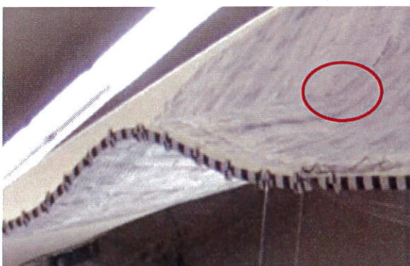
Sharp bend in the sandwich structure of the blade
