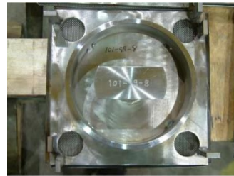
Figure 2-9. Damaged Fuel Can Lid with Screened Openings Photo courtesy of NAC International
