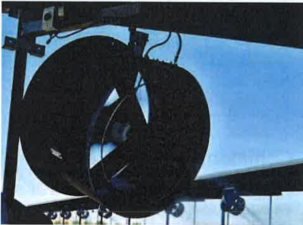
This is a 'Shade Tracker' evaporative cooling system in use on a farm in the US. This computerised system adjusts the amount of water output according to the temperature and relative humidity, and follows the shadow of the shade shelter through the day. This ensures that the cool air is always blowing into the shade.
