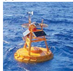
Floating met-ocean lidar system
