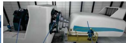
Nacelle equipment test platform
