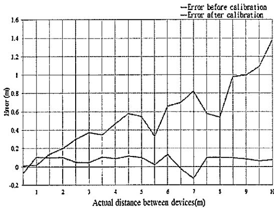
Figure 6. Calibration of localization error
