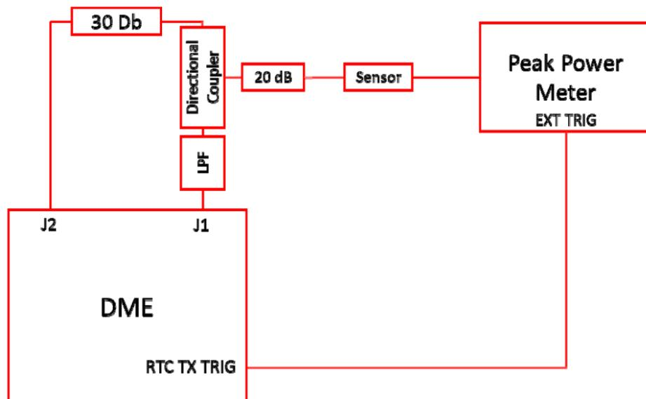
Figure 3-4 Transmitter Power Output Test Setup
