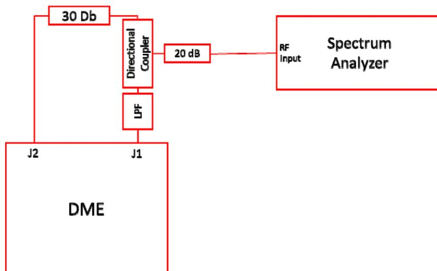
Figure 3-5 Spectral Characteristics Test Setup
