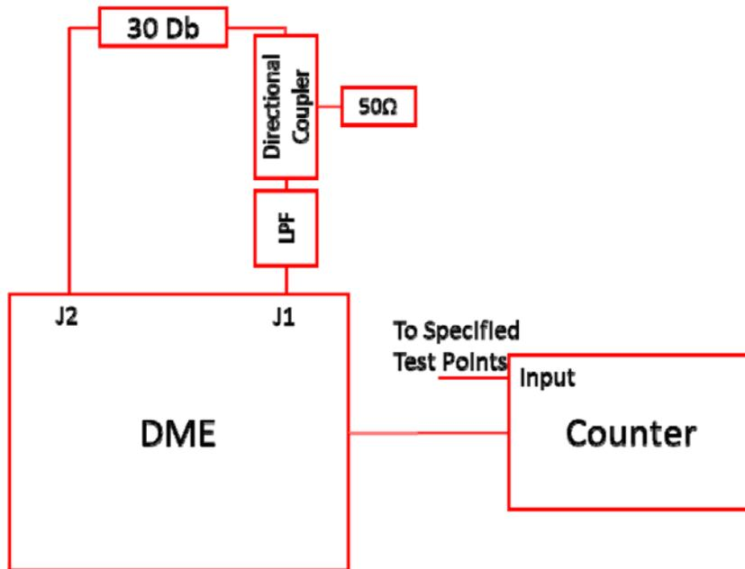
**Figure 3-3 Frequency Verification Test Setup**
