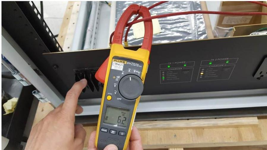
**NOTE:** The battery charge current will dip every five seconds as the BCSP is performing a battery fault test.
