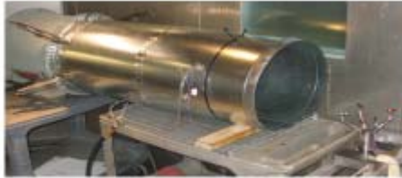
5400 CFM fan Honeycomb grid 1.2m long 50cm diameter Spray nozzle
