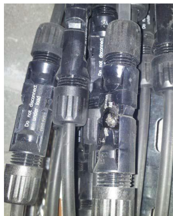
圖 8、DC connector showing a thermal event
