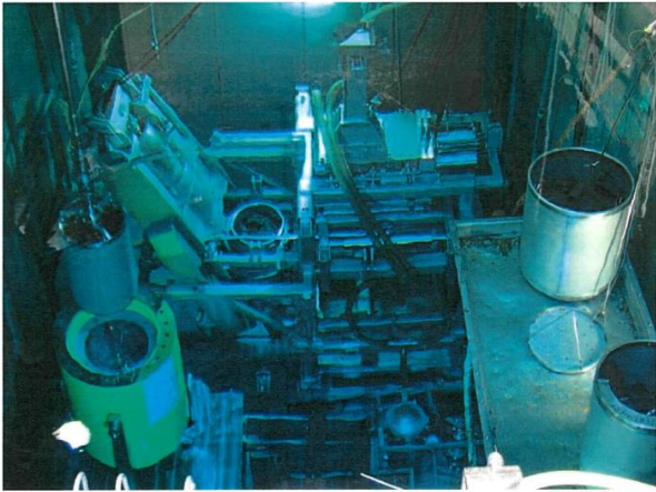
GNS Underwater Scrap Shears
