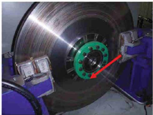
Picture 7: Measurement position at BS shaft end
