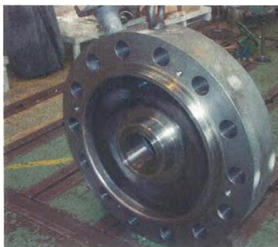
5.軸承外殼(Bearing Casing)
