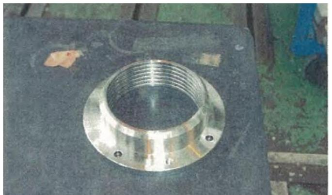
13.平衡套筒(Balance Bushing)
