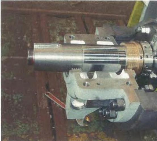
41.安裝驅動端下軸承外殼(inboard side)
