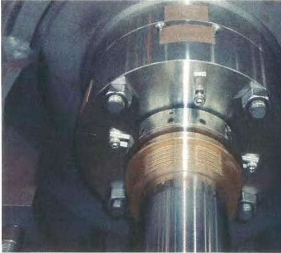
40.安裝機械軸封之套筒鎖圈(Sleeve Locking collar)及導流環(Deflector)
