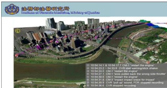
Figure 1.11-10 Superposing of GE235 flight path with an aerial photo and digital surface model during the last 23 seconds.
