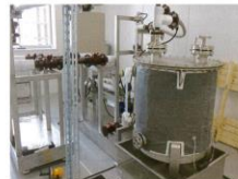
Examination device for hot spring system The device simulates a hot spring pipeline in the laboratory for evaluating hot spring monitoring sensors and conducting experiments on hot spring
