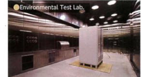
Environmental Test Lab. A large-size environmental test laboratory to conduct environmental tests such as a temperature and humidity cycle test, assuming use in desert areas, high-temperature and humidity areas, and very cold areas. It addresses a temperature range from -40°C to +80°C and a humidity range from 30%RH to 90%RH.
