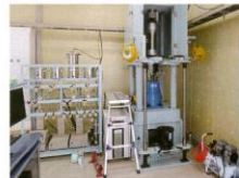
Experimental facility for shear slip of a fracture This facility enables the simulation of various mechanical phenomena in geothermal reservoirs under high temperature and pressure.
