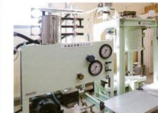
Experimental facility for the development of borehole tools for high-temperature and high-pressure geothermal wells This facility is capable of simulating 350°C, 60 MPa borehole conditions.
