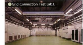
Grid Connection Test Lab.L The largest grid connection test laboratory in Japan accommodating a 20-foot-long container to conduct grid connection tests up to 3MW, and simulation power distribution line.
