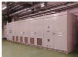
Grid Line Impedance 7km-long high-voltage power distribution line simulator for voltage fluctuation, etc.
