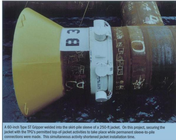
A 60-inch Type ST Gripper welded into the skirt-pile sleeve of a 250-ft jacket. On this project, securing the jacket with the TPG's permitted top-of-jacket activities to take place while permanent sleeve-to-pile connections were made. This simultaneous activity shortened jacket installation time.
