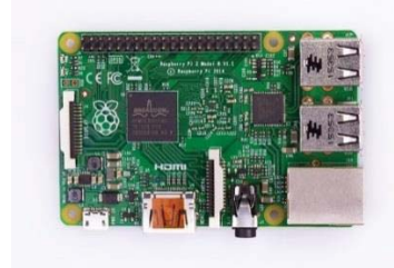
Figure 3. Raspberry Pi 2 Model B [8]
