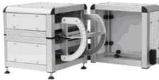
圖 12：BLA-1-limpness measurement device
