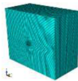
Figure 3. Mesh solution of the numerical model The overall model element mesh consisted of 1,173,872 EC3D8R elements.
