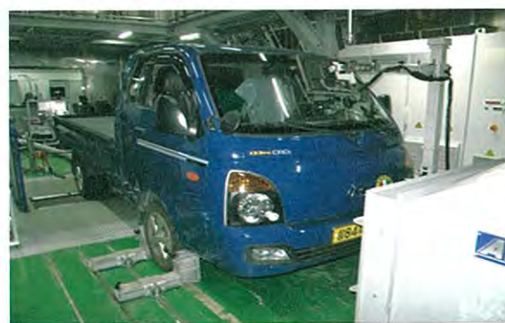
A system to measure emissions from light-duty diesel trucks
