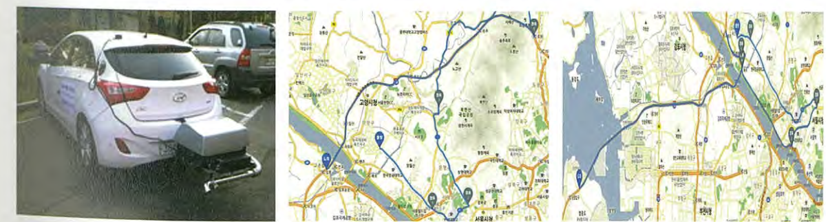
A test car equipped with PEMS and its driving test routes
