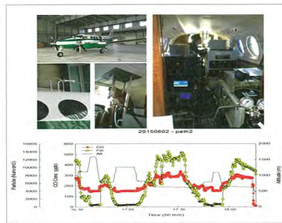
Airborne observation equipment and the measurement results
