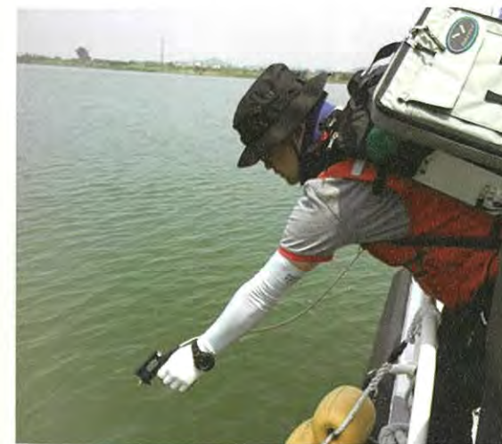
Measuring radiant energy from the water surface
