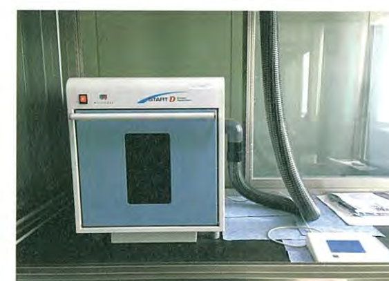
Heavy metal analysis using microwave acid digestion method
