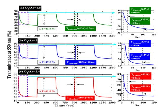
Figure 3 Temporal switching time characteristics between bleached states and colored states for the  $Ta_2O_5$  with electrolyte ECD for different relative ratio of oxygen and argon using applied voltages of +3.5 V (bleached state) and -4 V (colored state) while the duration time were fixed at 300 s (@550 nm). Inset Figure 3 (a) - (c), we are shown shortly duration time for 150 s
