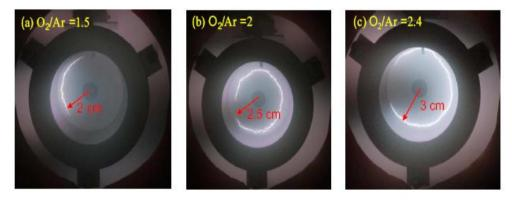
Figure 2 Schematic images of cathodic spotmotion under different relative ratio of oxygen and argon
