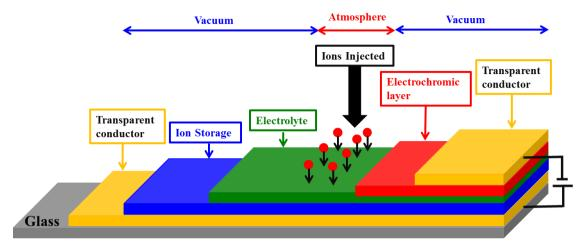
Figure 1. The typical structure of electrochromic device.
