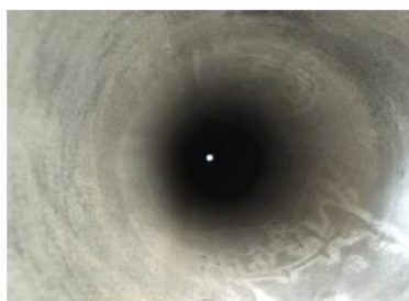
Helical tubes of different amplitudes and pitches with line of sight through the helical tubes
