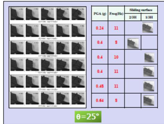
Sliding surface of the dip slope models
