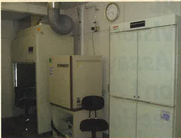
Safety Cabinet CO 2 Incubator Freezer (−30°C)
