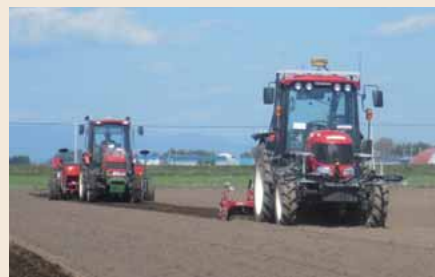
Collaborative work system that simultaneously performs two work operations with a driverless tractor and a tractor with a driver
